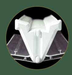
To provide a complete and tidy finish to any valley gutter, a 'clip on' extrusion has been designed. This new profile incorporates side wings that cloak the edges of the glazing bars and polycarbonate in the valley. A bespoke valley end cap totally conceals the lower end of the valley system, and is chamfered to match the end caps.
